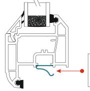
Fit a **BC001** Sash Spring to the sash on the center line of the stay fixing
