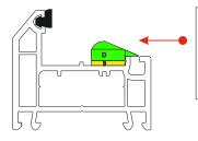
Fit a Frame Wedge "D" to include the packer "B" on the outer frame in the stay fixing area as shown
